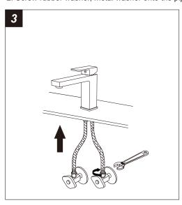
3.Connect the flexible hoses to water supply valve (not included) and copper tubes, and tighten it with adjustable wrench. DON'T OVER TIGHTEN!
